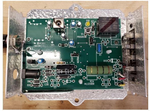
3. Connect the 412HM to your 12VDC power supply and plug that into 120VAC power. Pair your Car2U remote buttons(s) and/or the buttons on the remotes from your previous door operator with the 412HM. Pairing instructions are provided in the box with the unit. The photo above is of the circuit board inside the 412HM. An audible click from the relay (upper right corner of board above) when pressing a remote button paired with the 412HM confirms pairing success.
