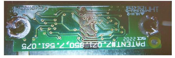
6. Solder a 10" pair of input leads to the circuit board's pushbutton pads, as shown below. This input circuit is a simple relay contact closure to translate a mechanical press of the button into an electrical voltage to the ADC circuitry, so it isn't necessary to maintain polarity end to end.
