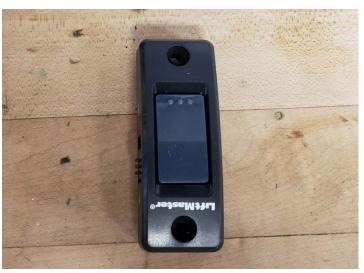
which contains a little board with circuitry to convert your button press into the correct digital pulse code for toggling your door's Open/Close operation.
