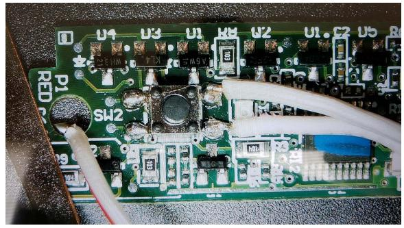
**NOTE:** I noticed that there wasn't enough solder on the button pads when I inspected the photo above, so I resoldered them.
