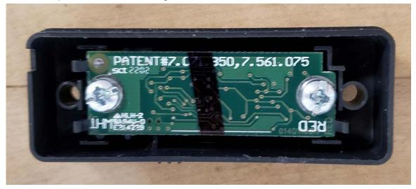
4. Completely remove the screws, and pry the circuit board out of the button housing. The component side of the circuit board is shown in the photo below
