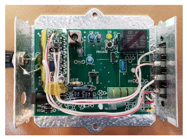
10. Re-label the screw terminals on the 412HM to indicate their new assignments. I used a Dymo labeler, but permanent marker would work fine. I also added a descriptive tag to the cover to alert service people that this unit is not stock. These additions are shown in the photos below
