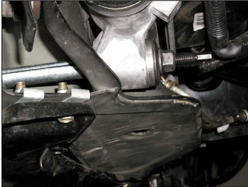
Figure 8 Installed MM aluminum steering rack bushing
