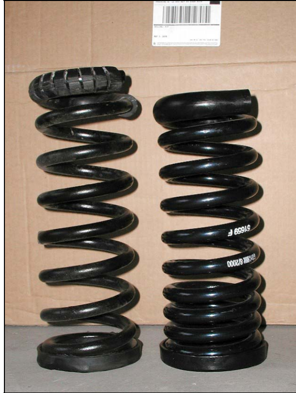
Figure 6 Front stock spring and isolators at left, H&R Super Sport w/ MM poly isolators at right (both inverted for balance)
