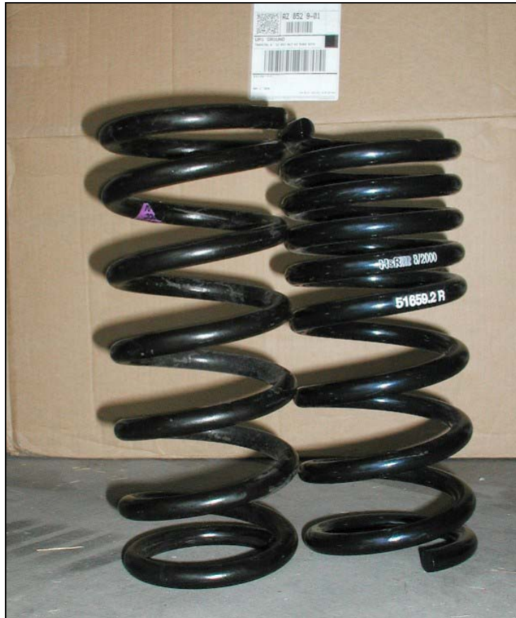
Figure 2 Rear stock spring left and H&R Super Sport right
