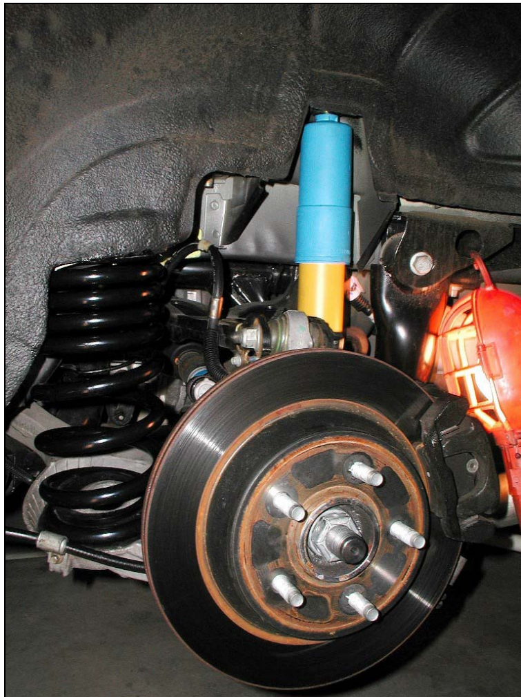
Figure 3 Driver side with new spring and shock installed
