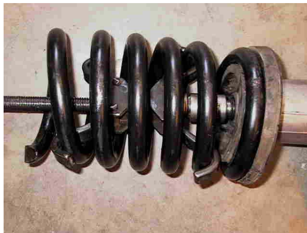
Figure 1 Stock rear spring on spring compressor
