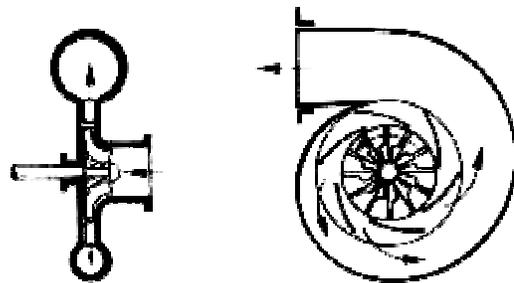
A centrifugal compressor needs rpm to make compression, boost falls off rapidly as rpm decreases. The compressor side works on the exact same principle as a turbocharger, only it's driven from a belt instead of an exhaust driven turbine. The centrifugal supercharger is more compact than the roots type and makes it much easier to use them in under the hood applications. They also work best as a blow through design.
