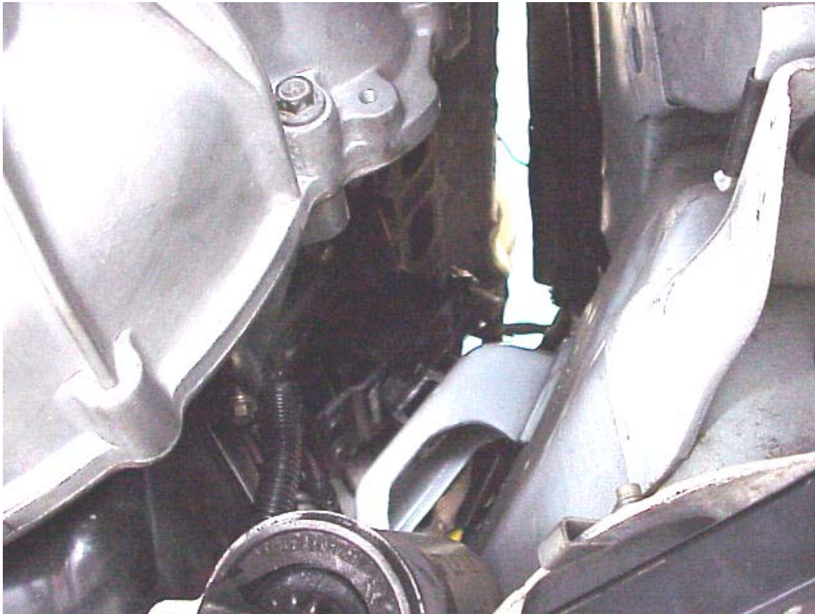
Figure 1 Passenger side of engine ready for header installation
