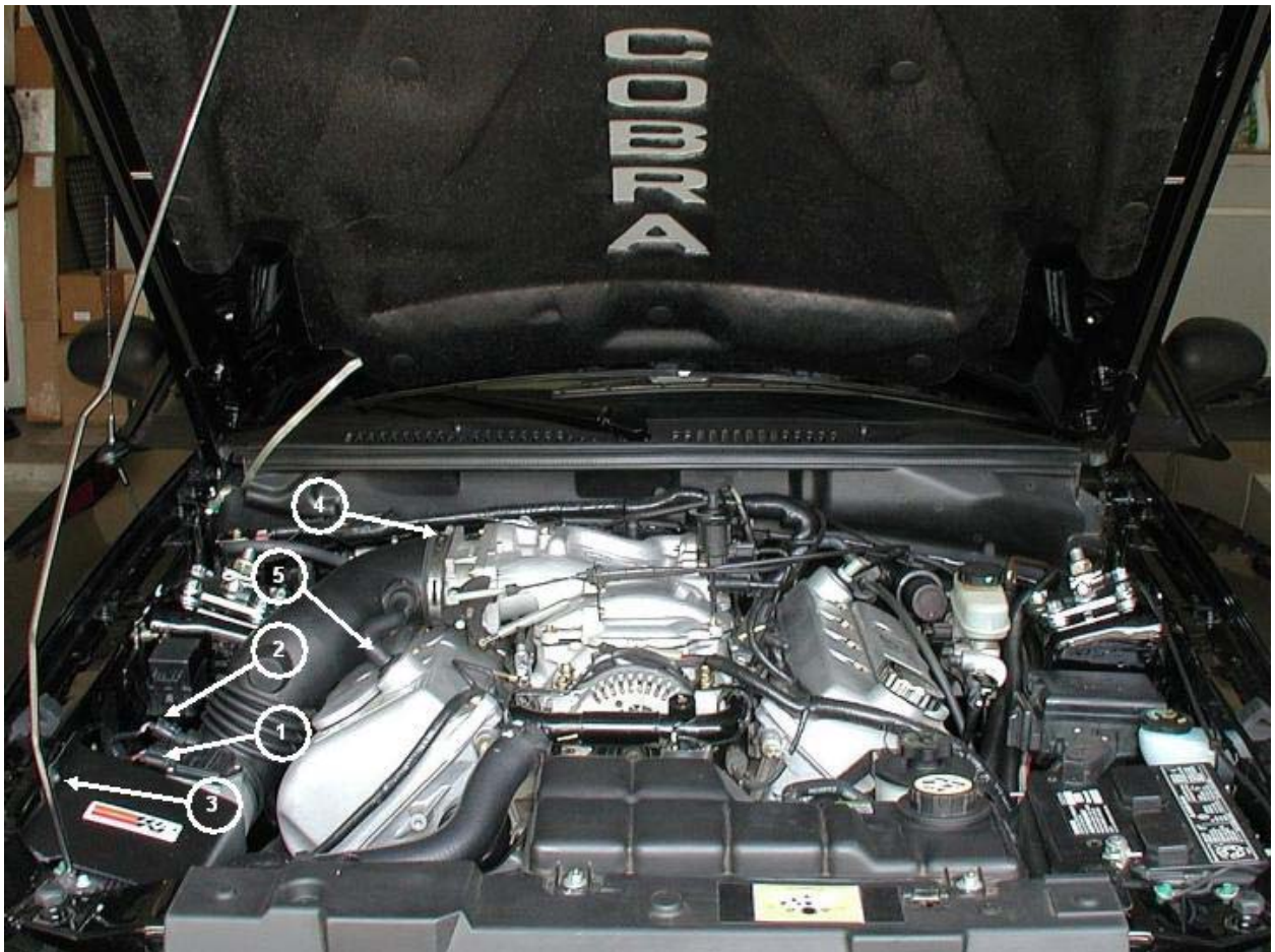
Figure 2 Engine Air Inlet Component Disconnection (aftermarket MAF, Filter, & Shroud shown)
