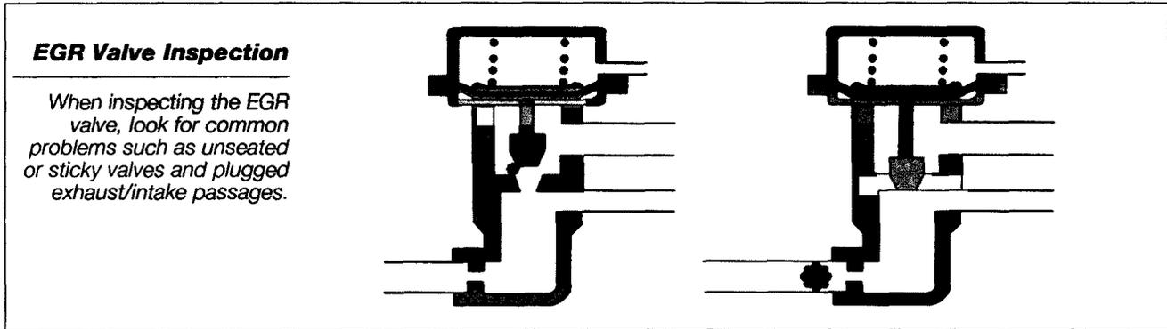
This inspection example systematically confirms the integrity of the EGR valve, VSV, backpressure modulator, system hoses, and EGR passages. Once the suspect part/component is identified, it should be individually tested and then repaired or replaced as necessary. Because slight model to model variations exist between EGR systems, refer to the Repair Manual for specific EGR system inspection procedures.
