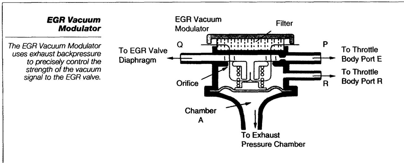
When vacuum is applied from port E, the strength of the vacuum signal applied to the EGR valve will be dependent on the amount of exhaust backpressure acting on chamber A of the vacuum modulator. When vacuum is applied from port R, the strength of the vacuum signal applied to the EGR valve will no longer be dependent on the strength of the exhaust backpressure signal. During this mode, the EGR signal strength is determined solely by
