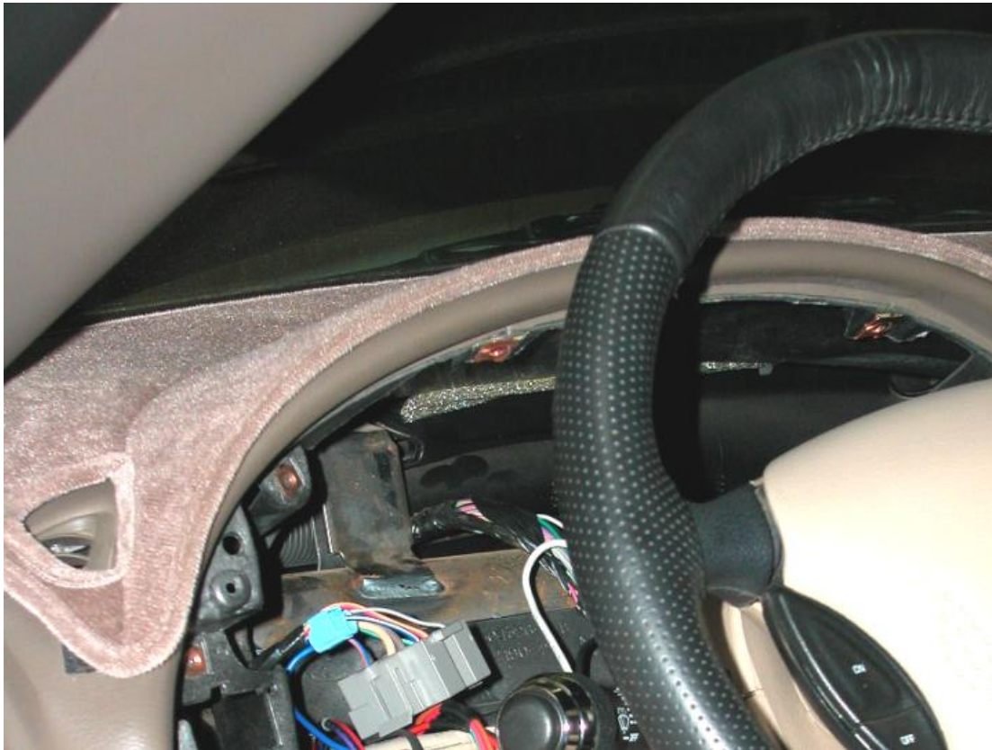
Figure 4 Gauge lighting circuit power tap
