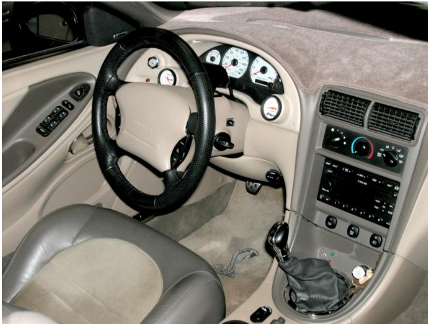
Figure 7 Completed gauge installation
